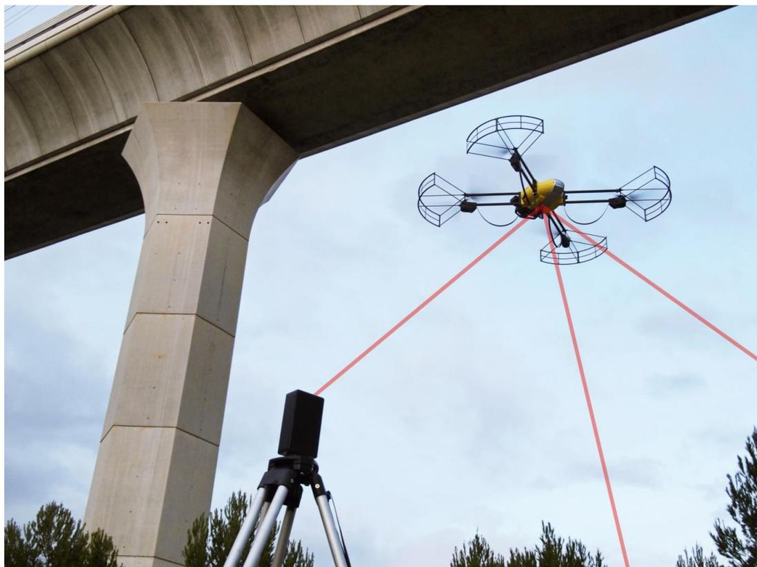
The NOVADEM U130 micro-UAV guided by the LPS technology performing an automatic inspection of infrastructure
